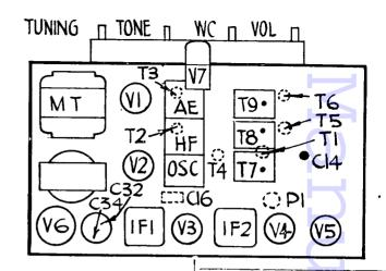
The model 319 covers two short wavebands and the medium band. In the circuit diagram below the coils are drawn with the medium wave circuits at the top. Trimmers are distributed both above and below the chassis.
