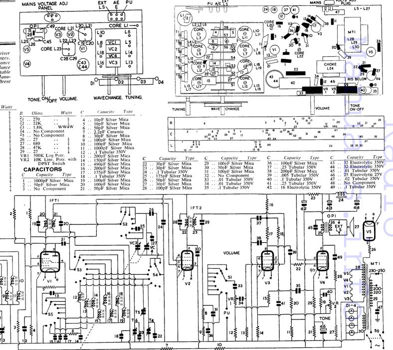
changer V1. S6 brings in the appropriate grid tuning capacitor VC2 or VC1. On LW and MW, and the 40-50m. band, VC2 is used; for the other SW bands VC1, shunted by C6, is employed. Bandspreading on the 40-50m range is obtained by connecting C9 in series with VC2, and on the other five SW ranges by use of the special VC1 which, on the 13, 16 and 19m bands, also has C10 connected in series with it.
